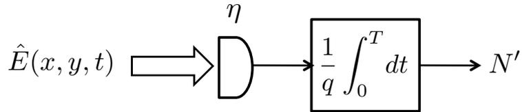
Figure 2: Sub-unity-quantum efficiency photon counter
