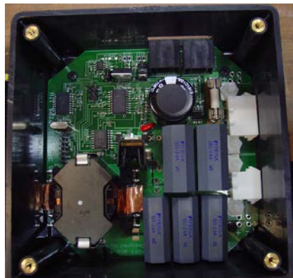
Custom "Boost Converter" MPPT tracker Developed by Robert Pilawa, MIT Solar Electric Vehicle Team
