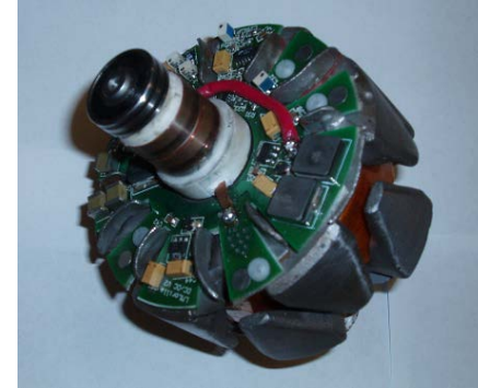
Foil field alternator with rotating power electronics MIT / LEES 2005
