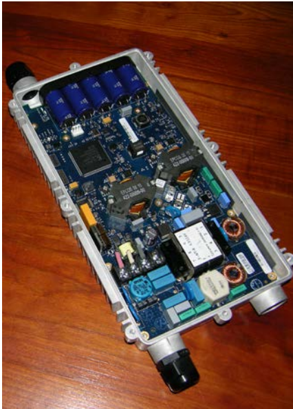
Microinverter for Photovoltaics Enphase Energy, 2008
