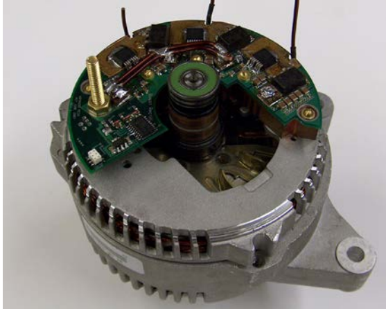
Alternator with Integrated Switched-Mode Rectifier MIT / LEES 2007
