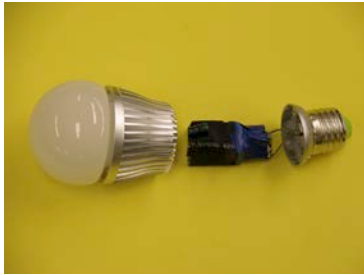
Efficient Lighting (LED driver)
