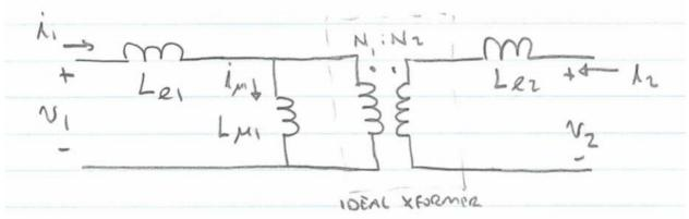
where:  $L_{l1}=\frac{N_1^2}{R_{l1}}$  and  $L_{\mu_1}=\frac{N_1^2}{R_c}$  and  $L_{l2}=\frac{N_2^2}{R_{l2}}$  and  $L_{11}=L_{l1}+L_{\mu_1}$  and  $L_{22}=L_{l2}+(\frac{N_2}{N_1})^2L_{\mu_1}$  and  $L_{\mu}=(\frac{N_2}{N_1})L_{\mu_1}$  So: leakage adds "independent inductance" in series with transformer leads! Both magnetizing inductance
