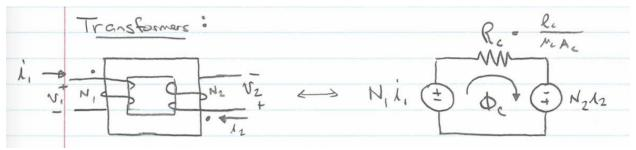
\* "Dot" convention: currents into the dots throw flux around the cone in the same direction.  $v_1 = \frac{d\lambda_1}{dt} = N_1 \frac{d\Phi_c}{dt} \qquad v_2 = \frac{N_2}{N_1} v_1$
