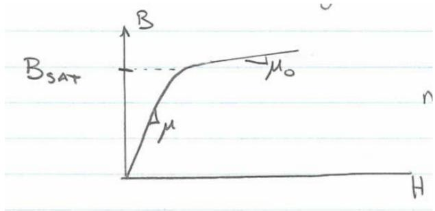
Above some flux density  $B_{\rm SAT},$  material saturates  $\frac{\delta B}{\delta H} \to \mu_0$
