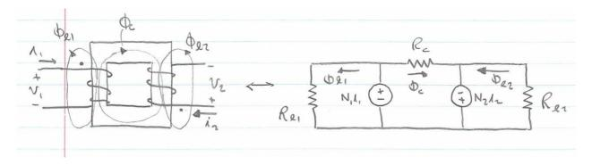
$$\Phi_{l1} = \frac{N_1 i_1}{R_{l1}}, \Phi_c = \frac{N_1 i_1 + N_2 i_2}{R_c}, Q_{l2} = \frac{N_2 i_2}{R_{l2}}$$
