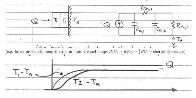
We can break the system down into as many lumps as needed. In limit, we can go to partical differential equation (distributed) representation.
