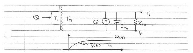
Note: This is a lumped parameter model for a distributed system. The temperature calculated is the average temperature across the block. If we want to look over short intervals of time (e.g.  $|| R_{th}C_{th})$ , at high frequency, or across small spaces, we need to use more "lumps".
