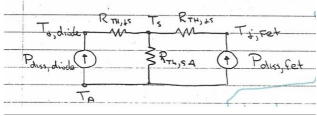
Dynamic case: If we have pulsed power (e.g. a UPS that runs for only a short time or a pulse discharge circuit that operates only once)
