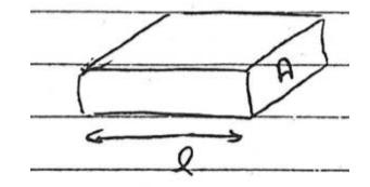
Because of this, we can connect thermal resistance and calculate temperatures + heat flows in various series and parallel paths using circuit model.
