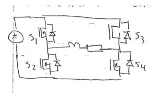
In VSI:  $S_1$  off <u>before</u>  $S_2$  on to avoid shorting  $V_{dc} \Rightarrow$  "dead time" <u>during which antiparallel diodes conduct</u>
