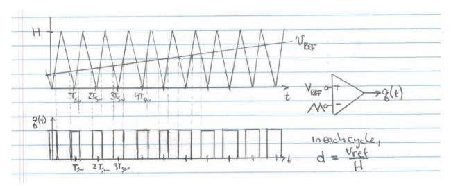
To get a bipolar output we could use one bridge leg to PWM synthesise  $|V_{ref}|$  and another bridge leg to "unfold" the output voltage (change polarity, etc).
