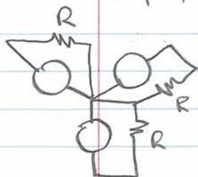
$$P_{TOTAL} = \frac{V_s^2}{R} \left[ \sin^2(\omega t) + \sin^2\left(\omega t - \frac{2\pi}{3}\right) + \sin^2\left(\omega t + \frac{2\pi}{3}\right) \right]$$
