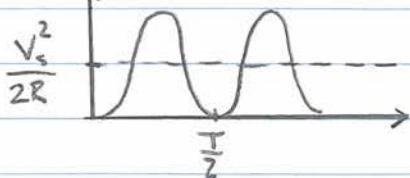
Even at unity power factor we get power pulsations between 0 and 2× average power at twice the line frequency. This makes sense, as we cannot draw power when  $V \rightarrow 0$ . This is bad for supplying power to machines, electronics, etc.
