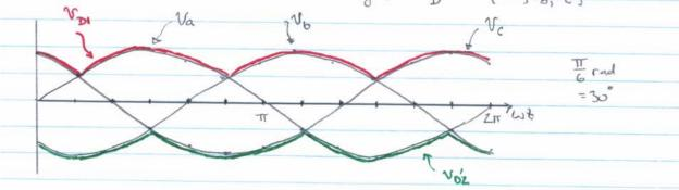
If we had <u>reversed</u> the diodes, we'd get  $v_{DZ} = min[v_a, v_b, v_c]$
