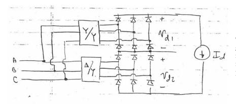
The  $\frac{Y}{Y_1}, \frac{\Delta}{Y}$  transformer sets generate equal voltage magnitudes, with a 30° phase difference between their 3 $\Phi$  outputs
