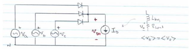
$v_D$  is the diode "or" of the three line-to-neutral voltages  $v_D = \max\left[v_a, v_b, v_c\right]$
