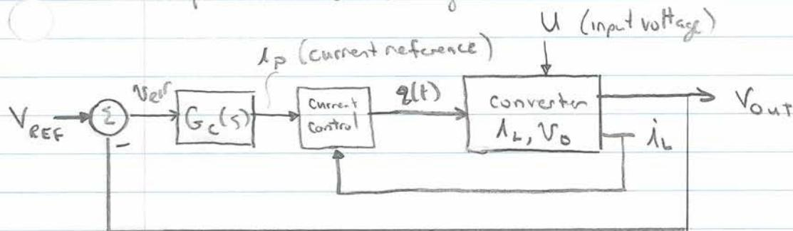
In peak current control we adjust the switching function  $q(t)$  such that
