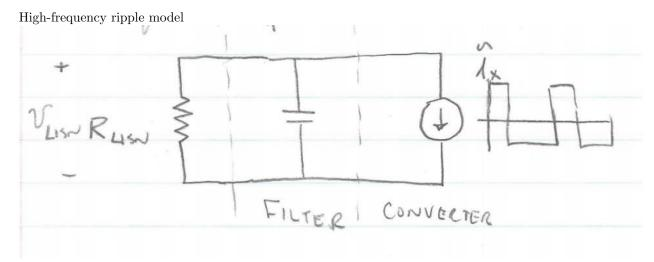
To achieve sufficient attenuation, a capacitor often insufficient. A higher-order filter is needed. The filter should pass dc current w low loss, and accept dc voltage with low loss
