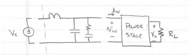
To regulate the output to a specified voltage (controlled) the converter needs to draw a certain amount of power from the input, independent of voltage  $v_i n!$
