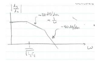
• high-frequency attentuation not as good as undamped  $L_f C_f$ . Move cutoff down to compensate.
