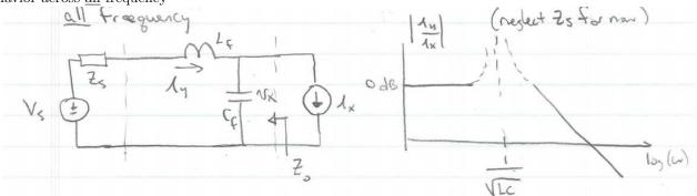
Neglecting  $Z_s$ , setting  $V_s \to 0$ , the converter looks back into a parallel LC tank circuit. At resonance, this becomes a high impedance + large resonant currents will flow!  $\Rightarrow$  must damp to be acceptable.
