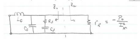
We require that the system remain well damped despite the tendency of the negative resistance to undamp the system.
