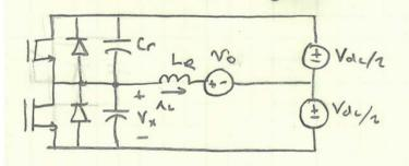
$\Rightarrow$  Overall operation:  $\langle i_L \rangle \approx \frac{i_{p+}+i_{p-}}{2}$ , e.g.  $i_f i_{ref} > 0, i_{p+} = 2i_{ref} + i_{min}, i_{p-} = -i_{min}$ Control  $i_{p+}, i_{p-}$  to achieve desired  $\langle i_L \rangle$  in a switching cycle. Also, there are requirements on  $i_{p+}, i_{p-}$  to achieve soft sw.
