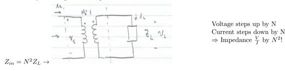
If we are concerned with sinusoidal waveforms over a narrow frequency range (as in resonant converters, RF communications, etc.), we can use a reactive matching network to effect impedance transformation.
