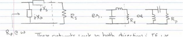
These networks work in <u>both</u> directions: If we transform <u>down</u> from  $R_p$  to  $R_s$  in one direction, we transform up from  $R_s$  to  $R_p$  in the other direction!
