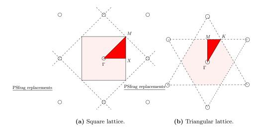
**Figure 2:** Irreducible Brillouin zones (red region) for (a) a square lattice and (b) a triangular lattice. Each region is defined between symmetry points of the crystal.
