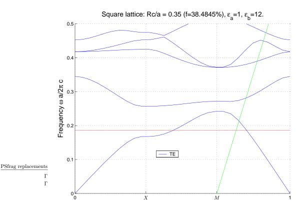
Figure 4: Band diagram for TE modes for the structure defined in Tab. 1. The horizontal line is at the frequency corresponding to a change of curvature of the k-surface, and the green line is the light-line shifted to M.
