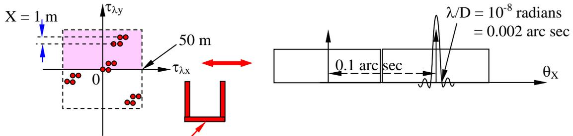
d) If the telescope apertures were square, we would need three rows of 50 telescopes arranged along three of the four sides of a field 50 m square, or perhaps in the shape of a tee, i.e., 150 telescopes. Since we probably are using circular apertures, the telescopes might be arranged more in the form of a circle, and the numbers might be reduced slightly.
