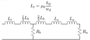
Figure 11: Equivalent Circuit: Double Bar
