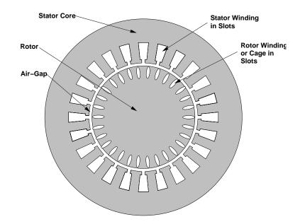
Figure 1: Axial View of an Induction Machine
