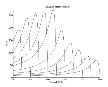
Figure 14: Induction Machine Torque-Speed Curves
