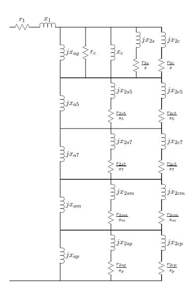
Figure 21: Extended Equivalent Circuit
