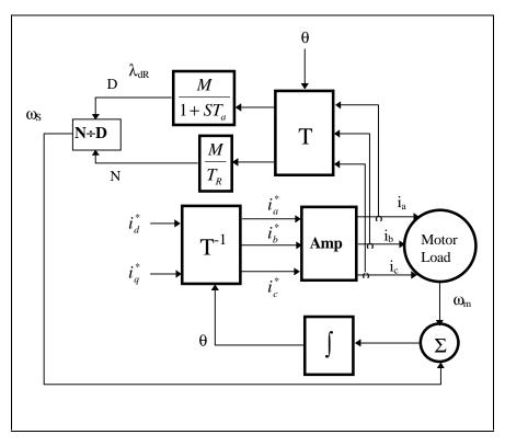
Figure 20: Field Oriented Controller
