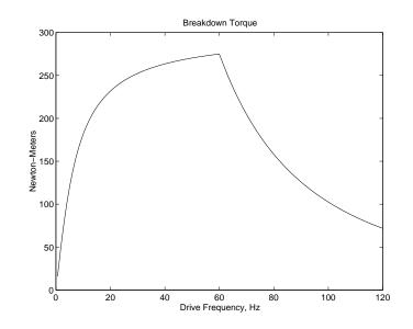
Figure 18: Torque-Capability Curve For An Induction Motor
