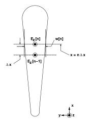
Figure 8: Slot Geometry Notation
