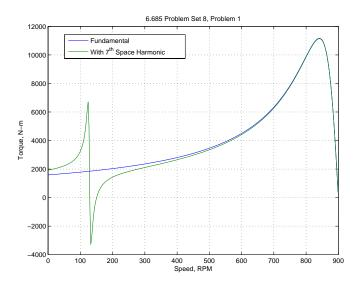
Figure 2: Torque-Speed with Seventh Harmonic
