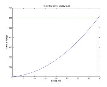
Figure 3: Voltage required vs. speed
