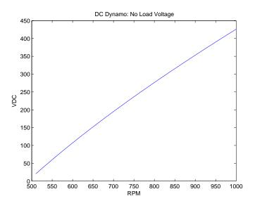
Figure 5: No Load Voltage
