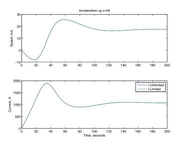
Figure 4: Simulation of Trolley Car Transient
