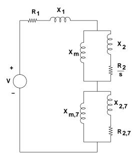
Figure 1: Induction Motor Equivalent Circuit with Seventh Harmonic
