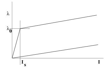
Figure 2: VRM Saturation Characteristic
