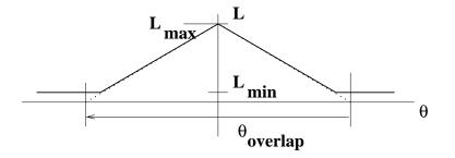
Figure 3: Inductance vs. Alignment Angle
