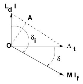
Figure 1: Vector Diagram for Torque Theorem Proof
