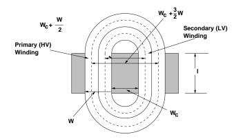
Figure 3: Winding Length Estimate
