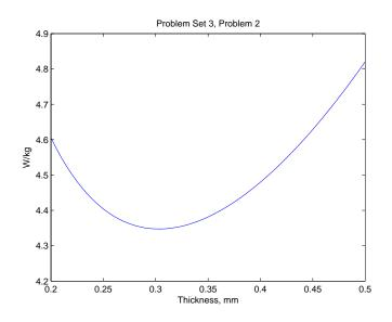
Figure 5: Loss as a function of sheet thickness
