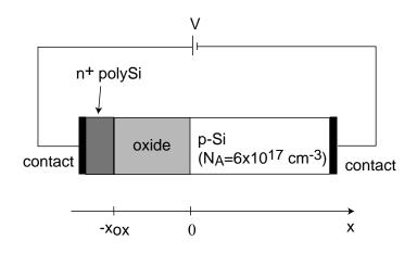
The oxide thickness is  $x_{ox} = 5 \ nm = 5 \times 10^{-7} \ cm$ . The gate is made out of n<sup>+</sup>-polySi with  $W_M = \chi_S = 4.04 \ eV$ .
