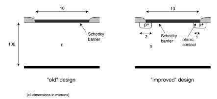
In both designs, the Schottky barrier height is 0.8 eV, the doping of the semiconductor is  $N_D = 10^{16} \ cm^{-3}$ , and the wafer thickness is 100  $\mu m$ . The ohmic contact to the body of the semiconductor is placed on the bottom surface of the wafer.
