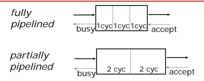
Function units have internal pipeline registers
