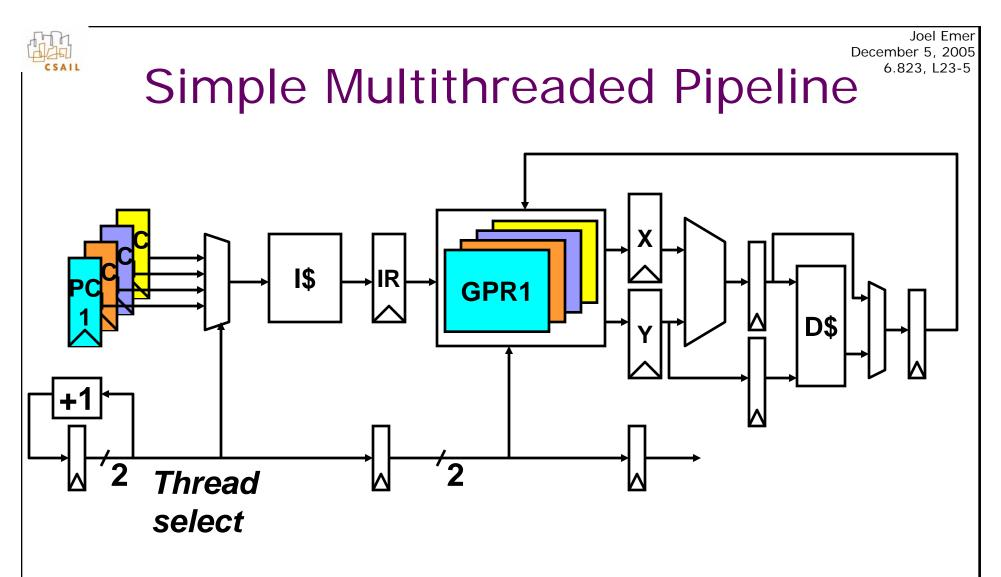
Have to carry thread select down pipeline to ensure correct state bits read/written at each pipe stage
