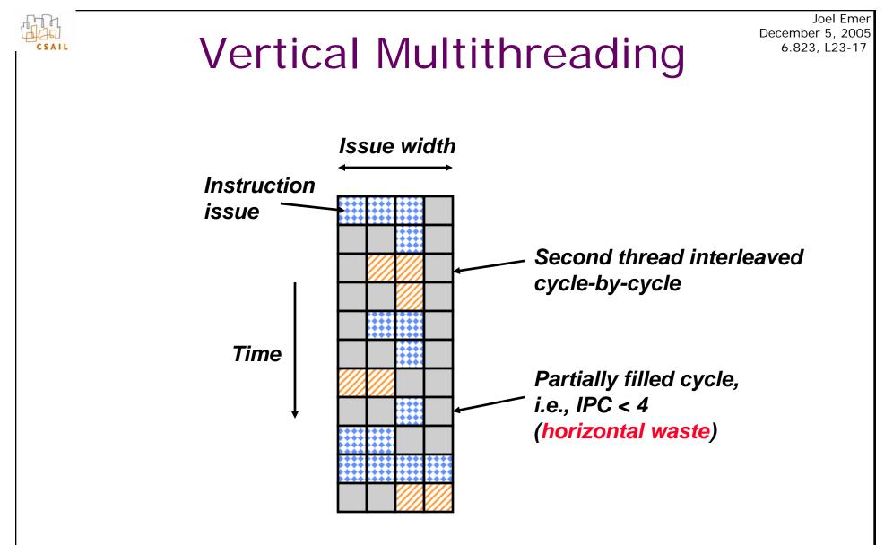
• What is the effect of cycle-by-cycle interleaving?
