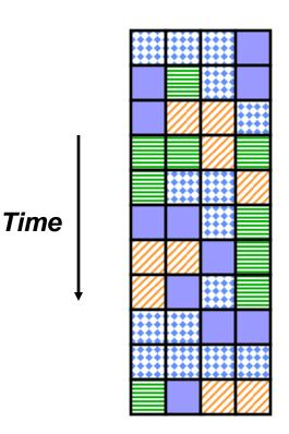
• Interleave multiple threads to multiple issue slots with no restrictions
