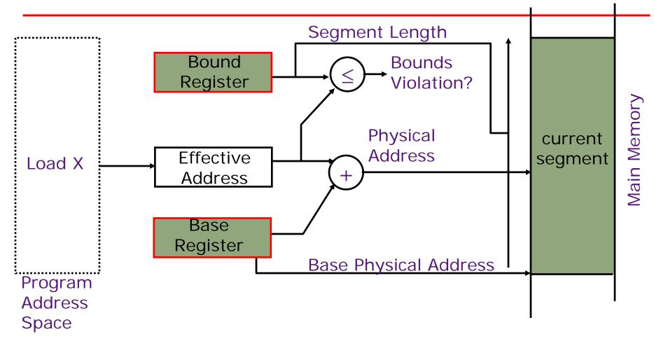
Base and bounds registers are visible/accessible only when processor is running in the *supervisor mode*
