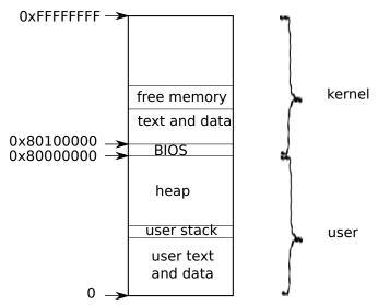
Figure 1-1. Layout of a virtual address space
