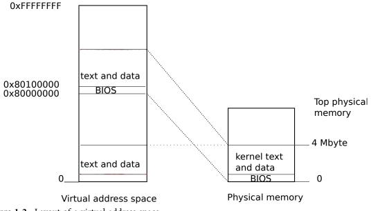
Figure 1-2. Layout of a virtual address space
