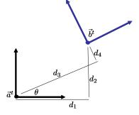
with distances given by the positive quantities  $d_i$ . What are the matrices R and T such that  $\vec{\mathbf{b}}^t = \vec{\mathbf{a}}^t T R$ ? Note: do this without using trigonometric terms in the matrix T. [/6]
