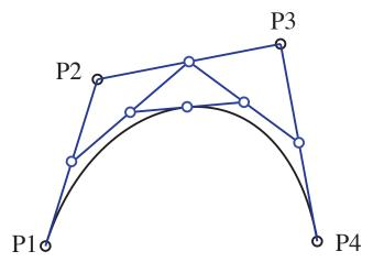
How can you choose the control points so that a cubic Bézier curve is a closed loop? [/4]
