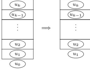
**Figure 3:** Change in the deque of a processor when the processor returns from a procedure.
