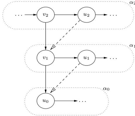
**Figure 8:** An augmented DAG corresponding to the execution DAG of Figure 9. The dashed edges have been added from continuation threads to spawn threads.
