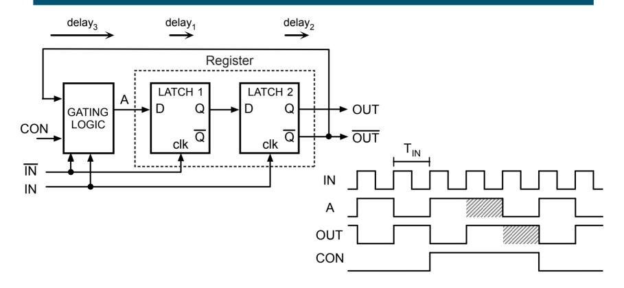
Maximum speed limited by latch plus gating logic
