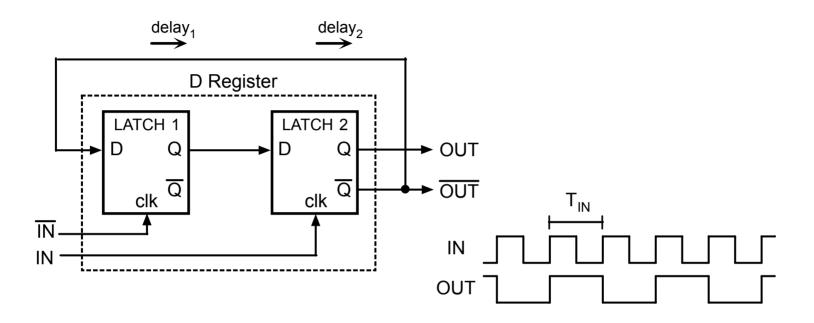
Maximum speed limited only by propagation delay (delay<sub>1</sub>, delay<sub>2</sub>) of latches and setup time of latches (T<sub>s</sub>)
