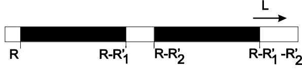
Figure 7.14: Transformed stability range for the four mirror resonator with R = (R_1 + R_2)/2 .
