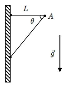
Two sticks are attached with frictionless hinges to each other and to a wall, as shown above. The angle between the sticks is  $\theta$ . Both sticks have the same constant linear mass density  $\lambda$ , and the horizontal stick has length L. Find the force (both horizontal and vertical components) that the lower sticks applies to the upper one where they connect at point A. Assume gravity points downward.
