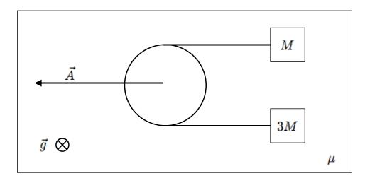
An idealized Atwood machine, consisting of a two blocks of masses M and 3M connected via a massless string through a massless pulley, sits on a flat horizontal table. The coefficient of kinetic friction between the block and table surfaces is  $\mu$ . The pulley is pulled by a string attached to its center and accelerated to the left. Assume that gravity acts with constant acceleration g down through the plane of the table.
