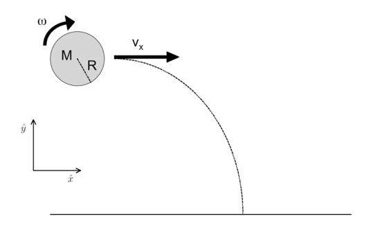
A superball of mass M, radius R and uniform density is thrown with horizontal velocity  $v_x$  and rotation rate  $\omega$  (assume that the spin angular momentum vector is orthogonal to the trajectory of the ball). The ball makes a perfectly elastic "bounce" on the floor without slipping, in a manner such that the magnitude of its vertical velocity is the same before and after the bounce (i.e., it would bounce to the same height from which it was originally released).
