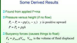
$\frac{V_{submerged}}{V_{object}} = \frac{\rho_{object}}{\rho_{fluid}}$
