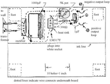
· black dot indicates wires soldered together
