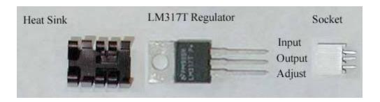
Figure 12: Heat sink, LM317T voltage regulator, and socket
