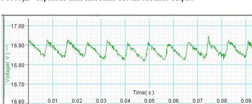
A  $1000 \mu F$  capacitor then smoothes out the rectifier output.
