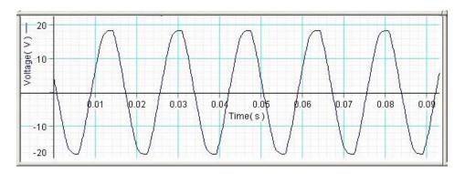
Figure 4: Wall transformer output voltage
