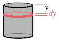
At a depth *y* the molasses pressure was  $p(y) = p_0 + \rho gy$ , where  $p_0$  is atmospheric pressure. If the tank had a diameter *d*, the area of the tank wall at *y* (a ring of height *dy*) was  $dA = (\pi d) dy$ . Force being pressure times area,
