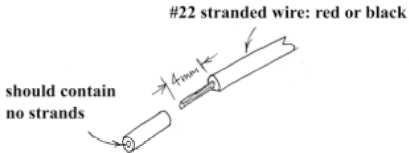
Figure 3: Stripping wires
