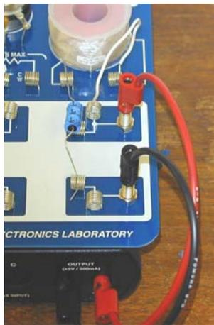
We will also again use the circuit board, set up with a 100  $\mu\text{F}$  capacitor in series with the coil (which serves both as the resistor and inductor in the circuit), as pictured at left.
