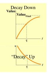
Interestingly, in RC & RL circuits any value that you could ask about (current, potential drop across the resistor, across the capacitor, ...) "decays" exponentially (either down or up). You should be able to determine which of the two plots at right a value will follow just by thinking about it. This reasoning forms the basis of most conceptual questions about DC circuits.
