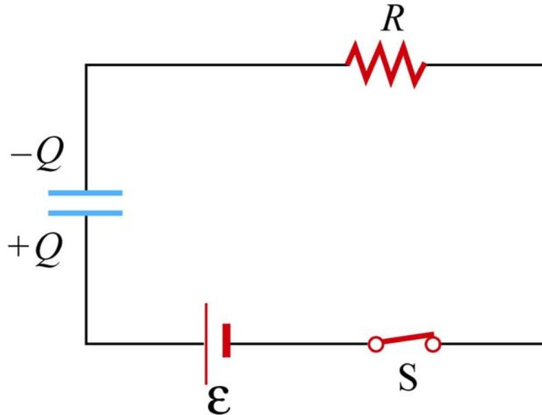
An uncharged capacitor is connected to a dc voltage source via a switch. A resistor is placed in series with the capacitor. The switch is initially open. At  $t = 0$ , the switch is closed. A very long time after the switch is closed, the current in the circuit is
