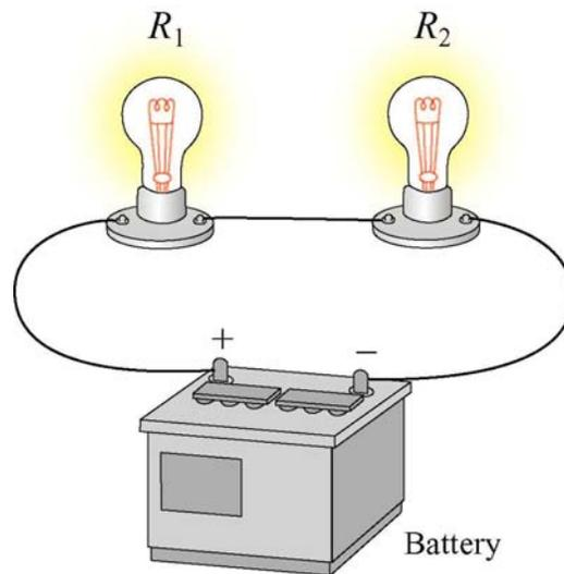
An ideal battery is hooked to a light bulb with wires. A second identical light bulb is connected in series with the first light bulb. After the second light bulb is connected, the light from the first bulb (compared to when only one bulb was connected)
