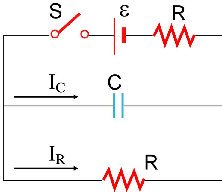
Consider the above circuit, with an initially uncharged capacitor and two identical resistors. At the instant the switch is closed:
