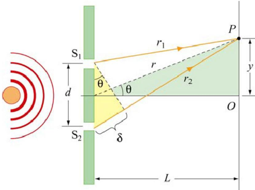
**Coherent monochromatic plane waves impinge on two apertures separated by a distance  $d$ . An approximate formula for the path length difference between the two rays shown is**
