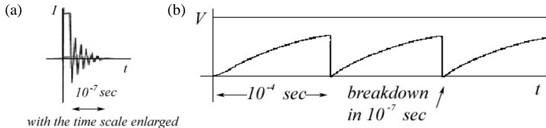
**Figure 2 Charging and Discharging the Capacitor.** The capacitor is slowly charged (limited by the RC time constant, with  $R = 4.5 \text{ M}\Omega$ ) and then (a) rapidly discharges across the spark gap, resulting in (b) a series of slow charge/rapid discharge bursts. This is an example of a “relaxation oscillator.”
