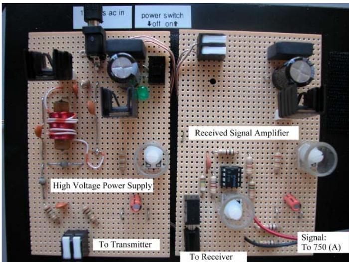
This board contains a high voltage power supply for charging the transmitter, as well as an amplifier for boosting the signal from the receiver. It is powered by a small DC transformer that must be plugged in (AC in). When power is on, the green LED (top center) will glow.
