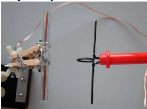
These have been described in detail above. The spark gap of the transmitter (pictured left) can be adjusted by turning the plastic wing nut (top). It is permanently wired in to the high voltage power supply on the circuit board. The receiver (pictured right) must be plugged in to the circuit board.
