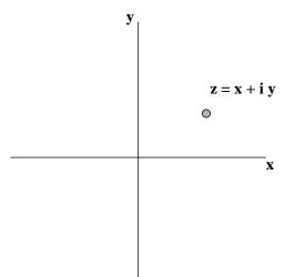
This is called the "complex plane" representation. Any complex number is given by a point in this plane. Using simple trigonometry, this point can be written in terms of a "magnitude"  $|z| = r = \sqrt{x^2 + y^2}$  and an angle or "phase"  $\theta = \arctan(y/x)$ :
