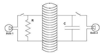
The current through the solenoid is turned on at t=0 and from that time has the form  $I_{\rm sol}(t)=\alpha t;\ \alpha>0$ . This current cycles counterclockwise (indicated by arrows). Both switches are open.
