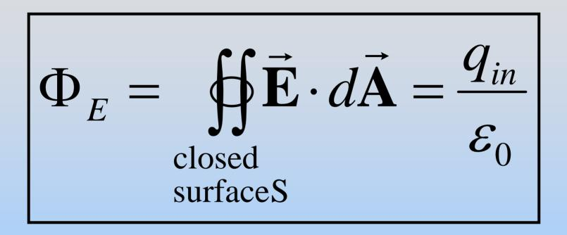
Electric flux  $\Phi_E$  (the surface integral of E over closed surface *S*) is proportional to charge inside the volume enclosed by *S*
