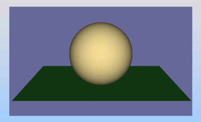
A rectangle is an open surface — it does NOT contain a volume A sphere is a closed surface — it DOES contain a volume
