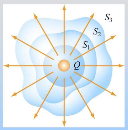
The total "flux" of field lines penetrating any of these surfaces is the same and depends only on the amount of charge inside
