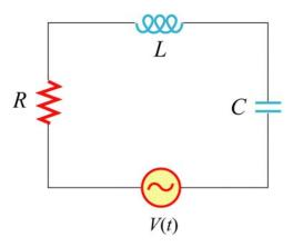
Figure 2 Driven RLC Circuit
