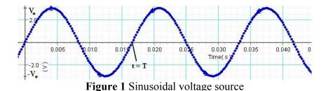
The sine function is periodic in time. This means that the value of the voltage at time t will be exactly the same at a later time t' = t + T where T is the *period*. The *frequency*, f, is defined to be the reciprocal of the period, f = 1/T. The units of frequency are inverse seconds, s<sup>-1</sup>, which are called hertz [Hz]. The angular frequency  $\omega$  is defined to be  $\omega = 2\pi f$ .
