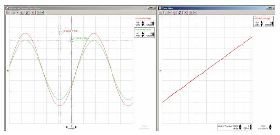
Figure 4 Waveform scope display (left) and phase plane scope display (right)
