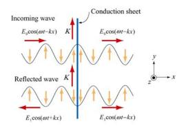
Figure 8 Idealized reflection from a conducting sheet
