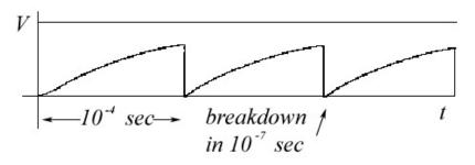
Figure 3 Breakdown Potential
