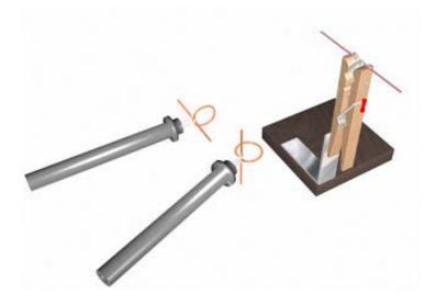
Figure 5 The spark gap transmitting antenna and the receiver
