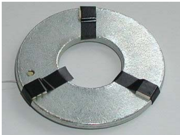
Figure 2: perf-board used as spacers on washer
