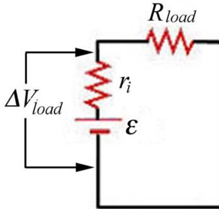
**Figure 9: Internal resistance of a voltage source**
