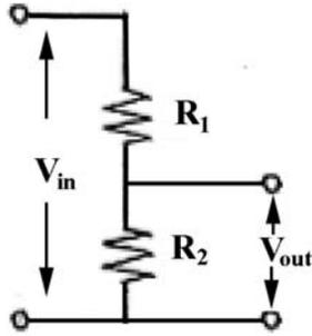
**Figure 8: voltage divider**
