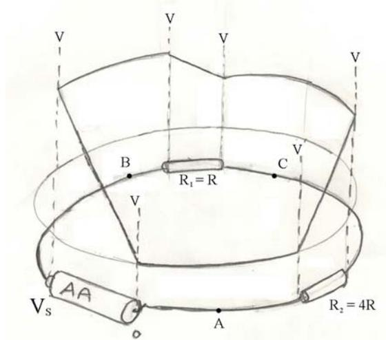
Figure 5a) Voltage changes around a closed loop
