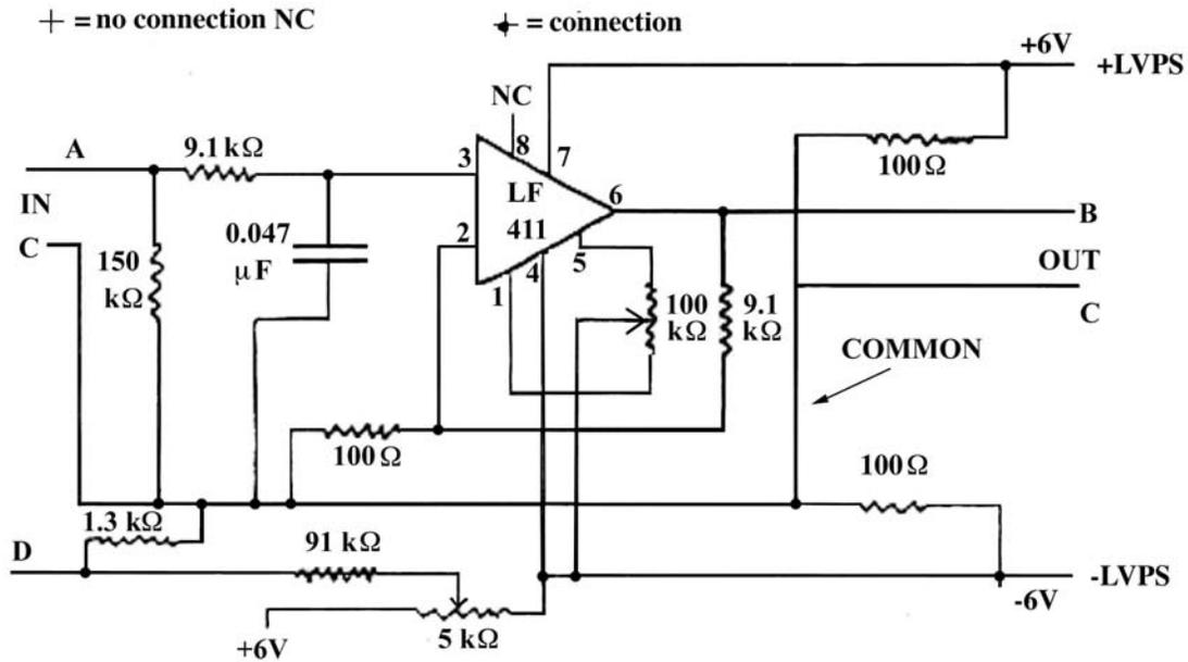
**Figure 1: Amplifier Circuit Diagram**
