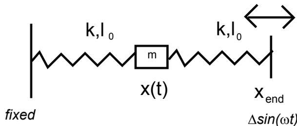
Figure 2: Classroom demonstration: mass on the air track
