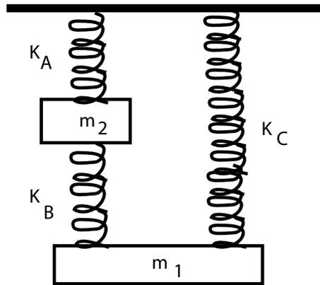
Figure 3: Two masses hanging vertically on springs
