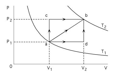
An ideal gas for which  $C_V = \frac{5}{2}Nk$  is taken from point *a* to point *b* in the figure along three paths: *acb*, *adb*, and *ab*. Here  $P_2 = 2P_1$  and  $V_2 = 2V_1$ . Assume that  $(\partial U/\partial V)_T = 0$ .
