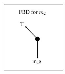
$$r_2 \ddot{\theta}_2 = \frac{\vec{F_2} \cdot \hat{\theta}_2}{m_2} \text{ or } \ddot{\theta}_2 = \frac{\tau_2}{I_2} = \frac{r_2(\vec{F_2} \cdot \hat{\theta}_2)}{r_2^2 m_2}$$
